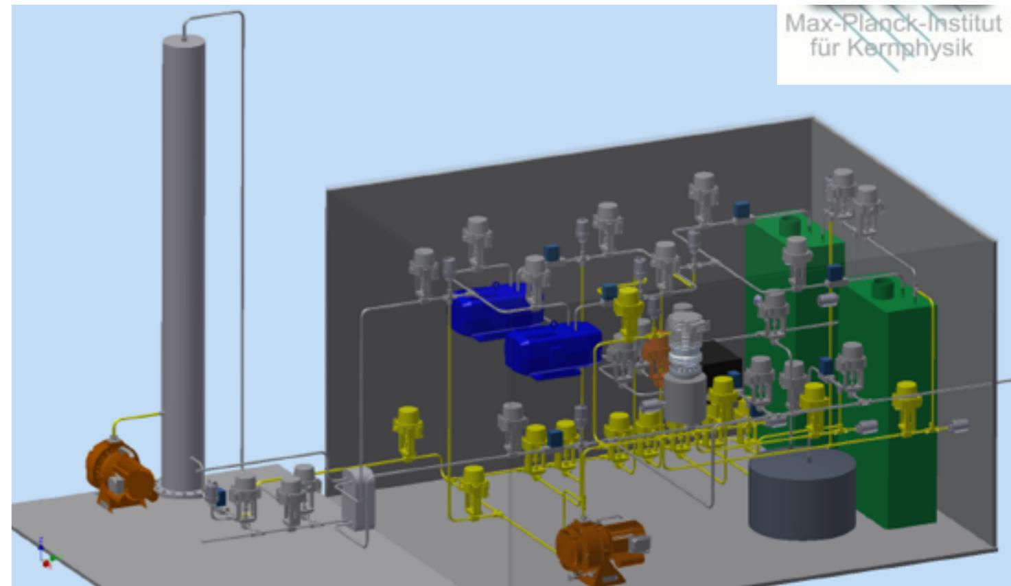
XENON1T purification loop with large charcoal tower.
