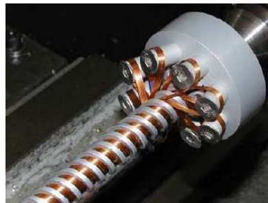
FIG. 9: (Color) Photo. winding of undulator showing return pegs to allow for continuous winding.
