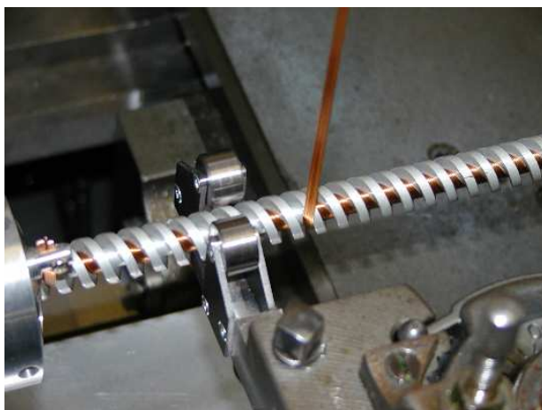
Figure 5.5: Undulator prototype with super-conducting (SC) wires being wound [199].
