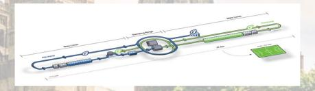
At 31km in length, the **ILC** will be the largest and also the most complex accelerator ever built. Besides the main linacs, damping rings with a circumference of 6 km for electrons and positrons are needed to produce the high quality beam required at interaction point. Physicists from all over the world participate in its design, but it is not yet known where the machine will be built.
