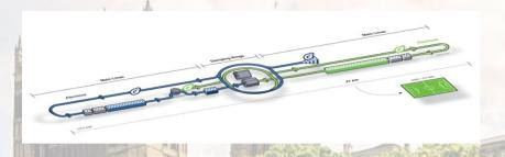
At 31km in length, the **ILC** will be the largest and also the most complex accelerator ever built. Besides the main linacs, damping rings with a circumference of 6 km for electrons and positrons are needed to produce the high quality beam required at interaction point. Physicists from all over the world participate in its design, but it is not yet known where the machine will be built.
