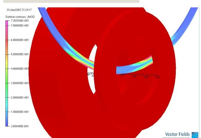
Above: Simulation of the eddy currents induced in the wheel by B-field Below: Power dissipated in eddy currents and torque
