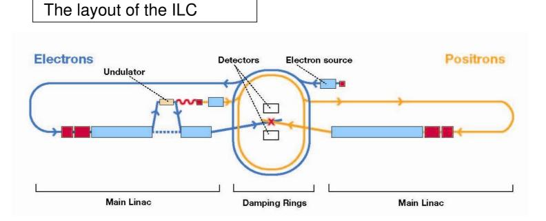
The helical undulator design has the strong advantage of producing the positrons in a longitudinally polarized state.
