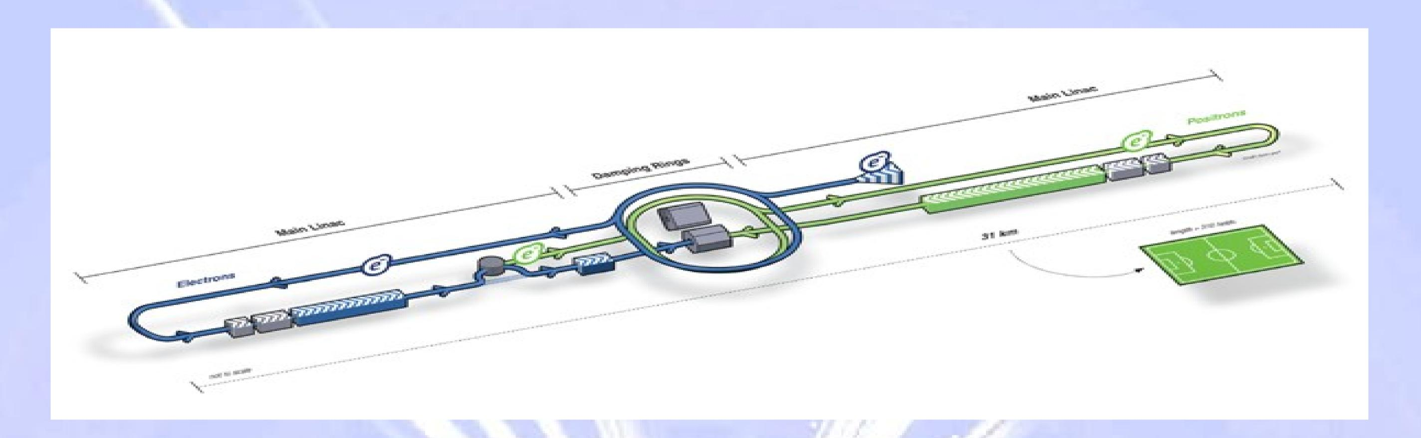
At 31km in length, the **ILC** will be the largest and also the most complex accelerator ever built. Besides the main linacs, damping rings with a circumference of 6 km for electrons and positrons are needed to produce the high quality beam required at interaction point. Physicists from all over the world participate in its design, but it is not yet known where the machine will be built.
