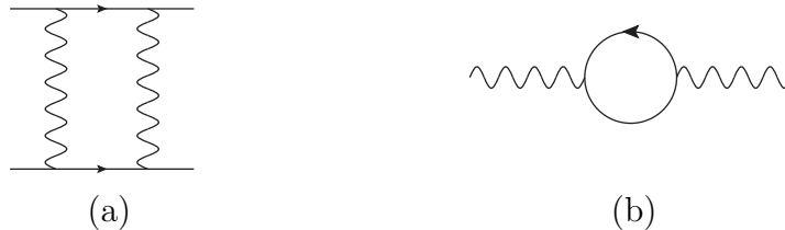
Figure 18: Sample “loop” Feynman diagrams: (a) one of the one-loop corrections to Coulomb scattering and (b) a one-loop correction to the photon propagator.
