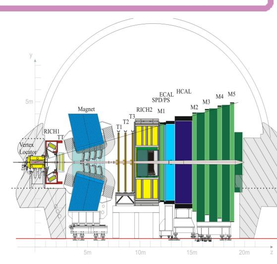
LHCb is characterized by excellent tracking and vertexing, particle identification system (good  $\pi$  – k separation capability), as well as a very good proper-time resolution and high trigger efficiencies, particular for muons.
