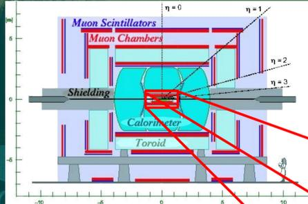
The D0 detector is a typical example of a collider detector, with tracking, calorimetry and muon systems. For this analysis, we make extensive use of the tracking and muon systems, but only limited use of the calorimeter.
