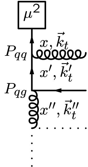
**Calculate  $f_q(x, k_t^2, \mu^2)$  by unfolding last step of evolution**
