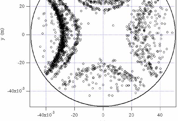
Particles in an accelerator can interact with each other and with their environment in many different ways. Some of the interactions can make the beam unstable: the beam size blows up, or the beam position jitters. Research and development are needed to make sure that effects such as electron cloud (*left*) in the positron damping ring do not limit the performance of the damping rings.
