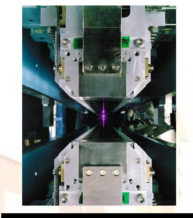
damping rates, are enhanced using superconducting "wigglers" (right) that generate very strong magnetic fields.
