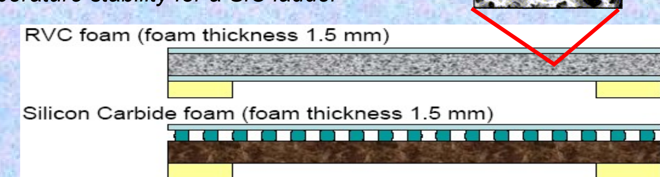
Layout of RVC and SiC ladders
