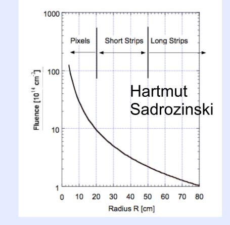
To maintain the resolution of the present ATLAS silicon tracking system we need:  $\rightarrow$  Finer segmentation
