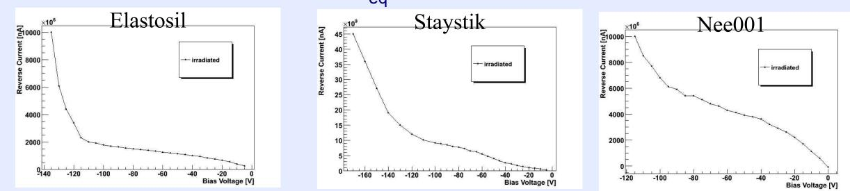
Measurements at < -40 °C show clear degrading for sensors glued with Staystik and Nee001, Elastosil leads to no differences in breakdown voltage
