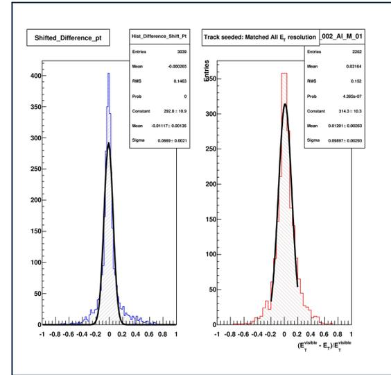
Figure 4: Transverse momentum resolution. Fast on the left in BLUE and full on the right in RED. Resolution is calculated by subtracting the  $p_T$  of a reconstructed tau that is matched to a truth tau from the  $p_T$  of the truth tau, all divided by the truth transverse momentum. Black line on both plots is a Gaussian fit, parameters of which are shown in the key.
