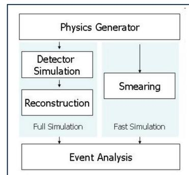
Figure 2: Flow chart representing fast and full simulations.
