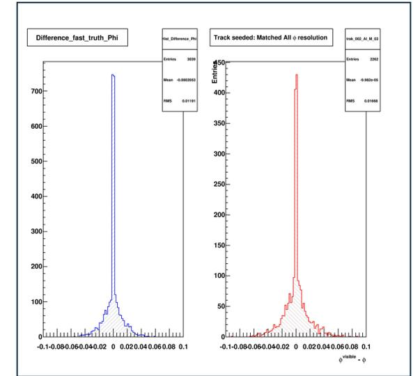
Figure 5: Phi Resolution, same colour scheme as figure 4. Resolution is here calculated by subtracting reconstructed and matched tau phi from truth tau phi.
