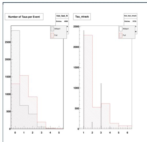
Figure 3: Comparison between fast and full simulations. Left hand plot shows number of taus per event, right hand plot shows (normalised to same number of taus) tracks per tau.
