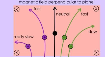
The curvature of a particles track is proportional to its velocity and momentum. The direction of the curvature shows the charge of the particle.
