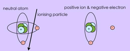
The transferred energy from the incoming particle to the shell electron allows the electron to overcome the binding forces to the atomic core. Neutral particles cannot be detected in the tracking detector as they do not interact with the shell electrons of the atoms.
