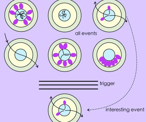
A scintillator is a material emitting light when an energetic particle passes through. This is one possible detector for fast triggering.
