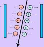
By measuring the drift time for electrons between track and anode, the spatial resolution can get even smaller than the sensor size.
