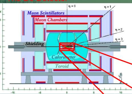
The muon system is composed of three layers of scintillator tiles and drift tube detectors. A toroid between the 1<sup>st</sup> and 2<sup>nd</sup> layers curves the muon tracks aiding in momentum determination. Hits in the muon layers are used to trigger the detector. The toroid polarity is reversed on a regular basis allowing the determination of the detector asymmetry separate from the CP asymmetry.
